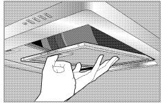
10. Install the carbon filter as per the following figure.
