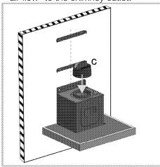
6. For chimney connection usage: In chimney connection installation, the absorbed air will pass through the aluminium filters and will be expelled to the outside through the connection pipe.
