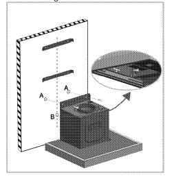
5.As shown in the figure below, place the cover (C) -that prevents reversed air flow- to the chimney outlet.
