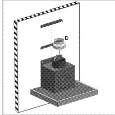
When this connection position is used, chimney connection adapter D is placed on part C as shown in the figure above.
