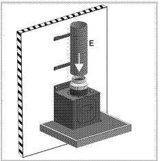
You should make sure that the chimney connection pipes used are made of fireproof plastic material. When using flexible connection pipe, it should be considered that sharp corners and sudden contractions will have a negative impact on air suction.
